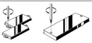
\*Instruments that have adjustable pole pieces can be adjusted to balance the output of each string.
